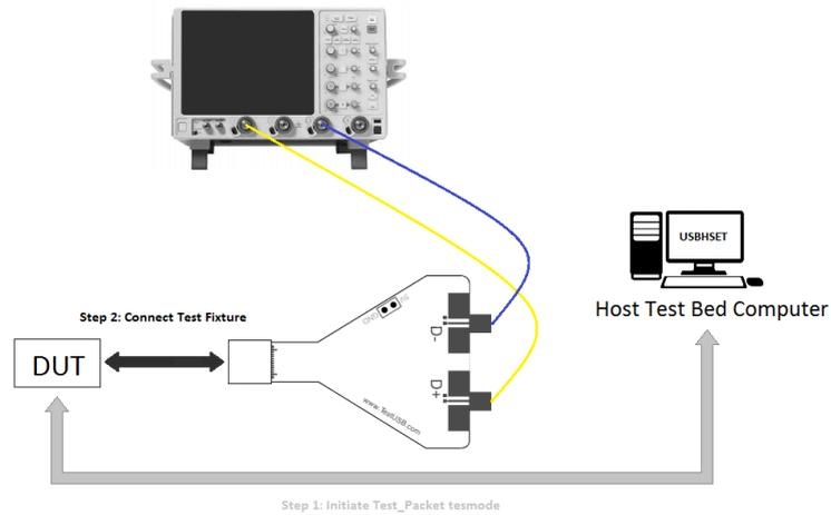
Connecting the Equipment – DUT has Type-C™ receptacle and is self-powered (Test fixture FS-HUCP)
