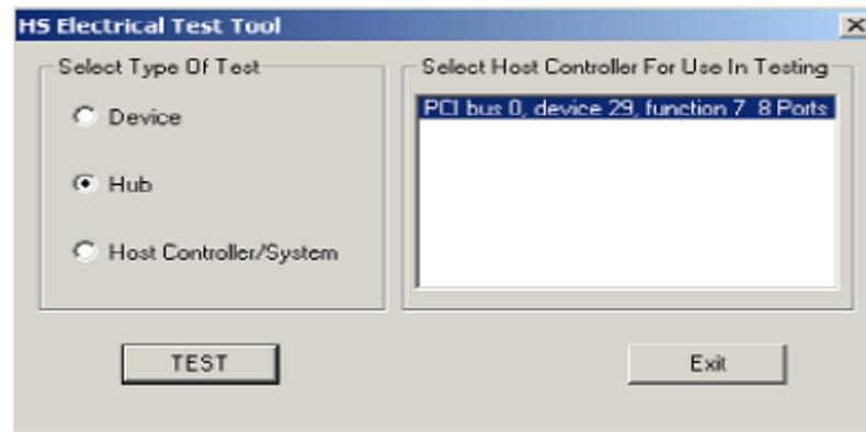
5. The hub under test should be enumerated with the device's VID shown together with the root port in which it is connected.
