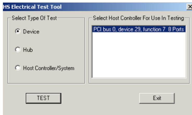
11. The device under test should be enumerated with the device's VID shown together with the root port in which it is connected.
