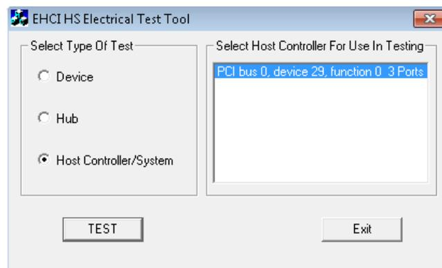
8. The Host Test menu of the HS Electrical Test Tool should appear as below.
