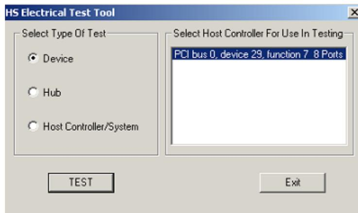
3. The device under test should be enumerated with the device's VID shown together with the root port in which it is connected.
