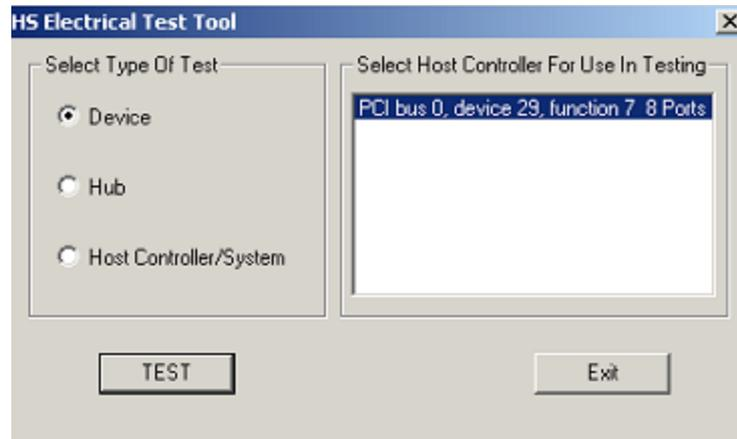
7. The device under test should be enumerated with the device's VID shown together with the root port in which it is connected.
