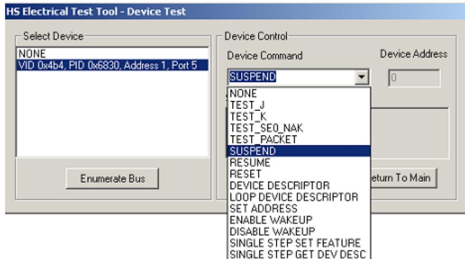
19. On the Device Test Menu of the HS Electrical Test Tool, select **RESET** from the Device Command drop down menu. Click **[EXECUTE]** once to reset the device operating in high speed.
