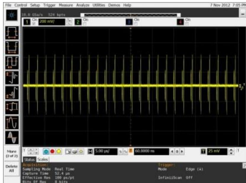
11. When the DUT respond with NAK to all 12bit Sync packets the test is PASS.
