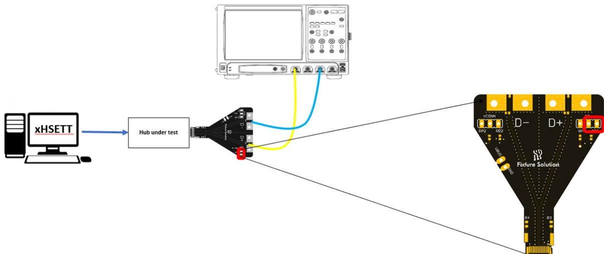
1. Connect the Hub under test upstream port to the Test Bed Computer running xHSETT, using a USB cable.
