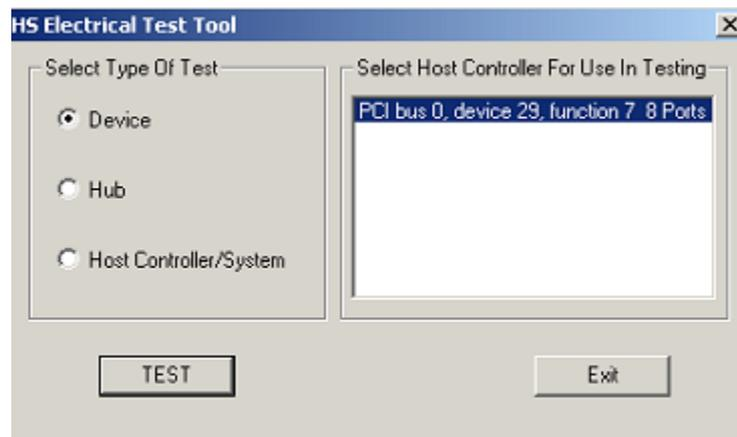
8. The device under test should be enumerated with the device's VID shown together with the root port in which it is connected.
