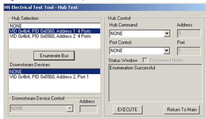
11. On the Hub Test menu of the HS Electrical Test Tool, select SINGLE STEP SET FEATURE from the Downstream Device Control drop down menu and click [EXECUTE] once.
