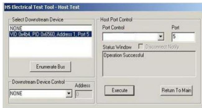
(If the hub is not visible it might be possible you need to flip the Type-C cable at DUT 1 or Host init 1 side)
